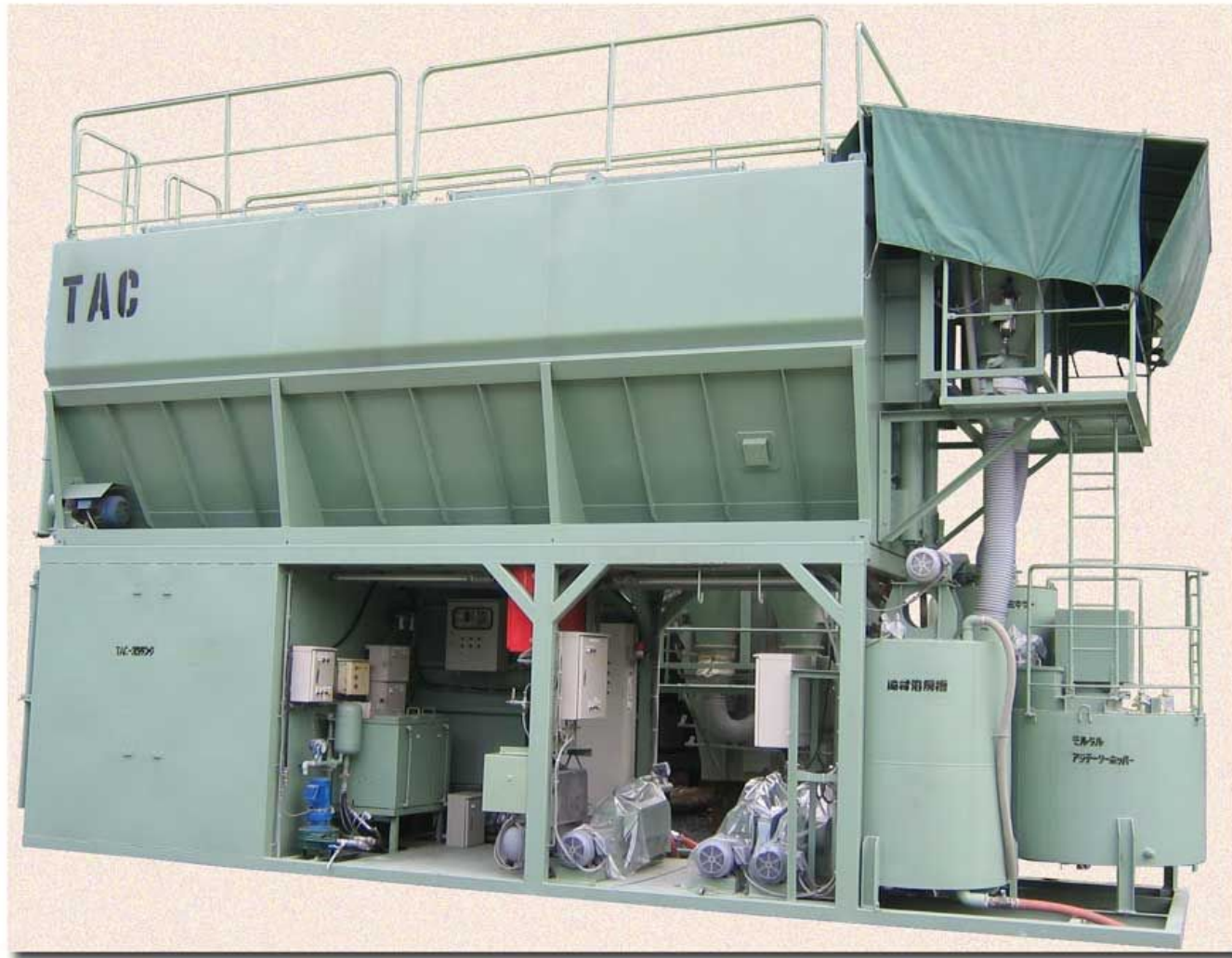
Automatic Plant for Backfill grout & Additive Injection
